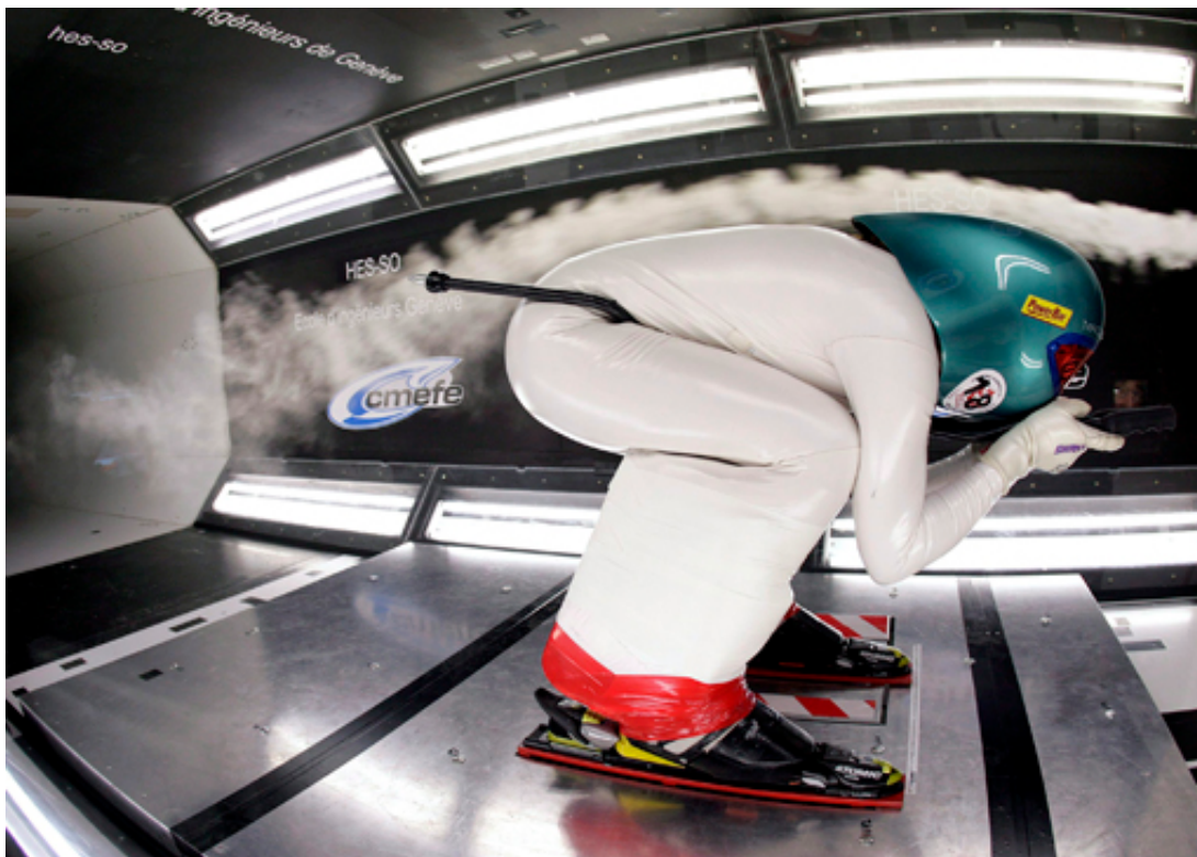
Figure 7 A speed-skier inside a wind tunnel. The white smoke shows the flow of air over the speed-skier's body.
