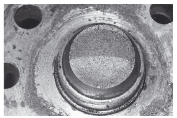
Figure C17 Brittle fracture in cast-iron
