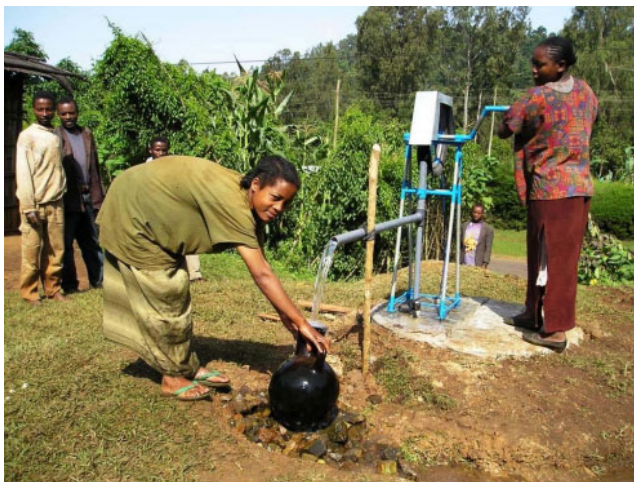
Figure 6.2 A hand-dug well with rope pump: an appropriate technology for rural supply because it is simple to operate and maintain, affordable, reliable, and can be locally manufactured.
