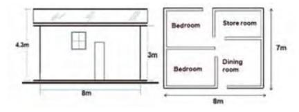
Figure 4.3 A housing unit with corrugated iron sheet roof and its floor plan.
