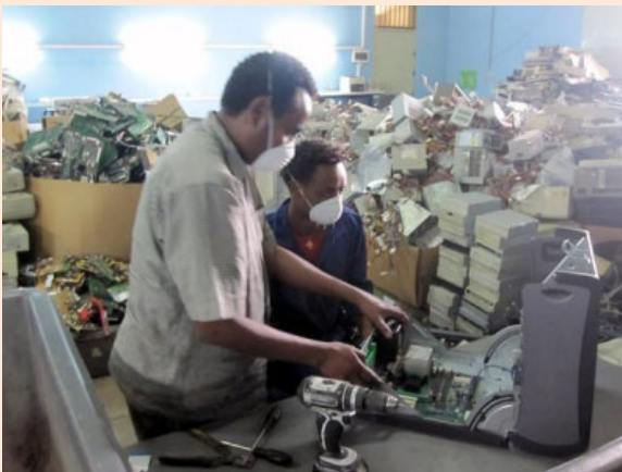
Figure 1.10 Computer dismantling in the Demanufacturing Facility in Akaki, Ethiopia.
