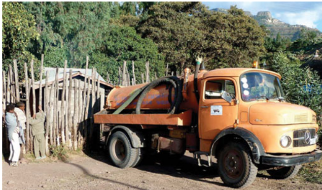
Figure 6.5 Streets in urban areas need to be wide enough to allow access for sludge tankers.
