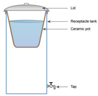
Figure 10.7 Ceramic pot method of water filtration.
