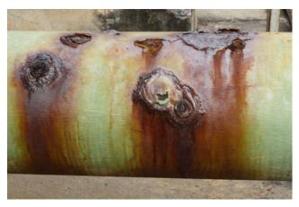
Figure 7.4 A section of corroded water pipe.
