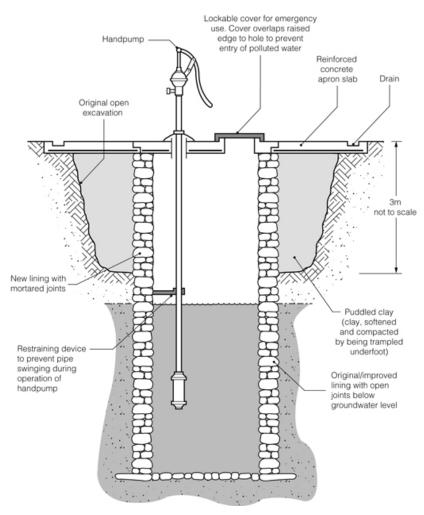
Figure 3.4 Diagram of a hand-dug well.
