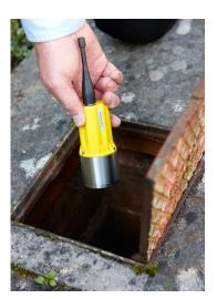
Figure 7.6 An acoustic logger to detect leaks through a change in noise level in the water pipe.
