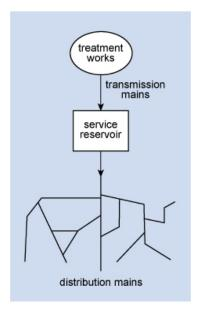
Figure 1.10 A simple water distribution network.
