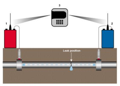
Figure 7.5 A noise correlator system to pinpoint the location of a leak.
