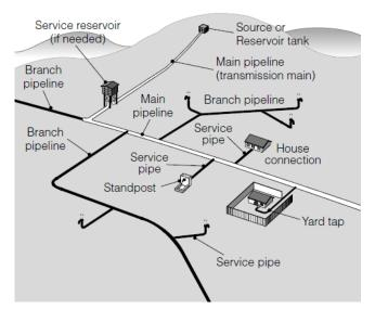
Figure 7.1 Schematic of a water distribution and delivery system.
