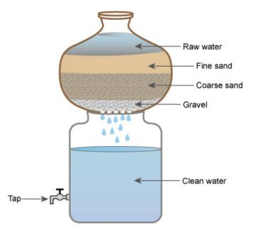
Figure 10.6 A household sand filter system, comprising a pot and a storage vessel.
