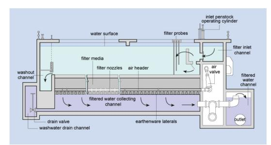
Figure 5.7 Cross-sectional diagram of a rapid gravity sand filter.
