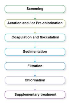
Figure 5.2 The seven steps often used in the large-scale treatment of water.
