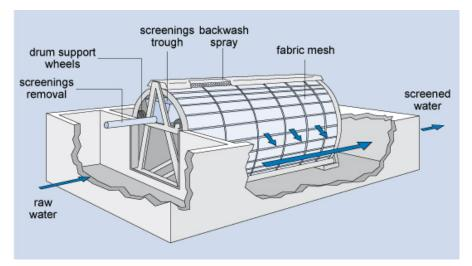
Figure 5.4 Diagram of a microstrainer.
