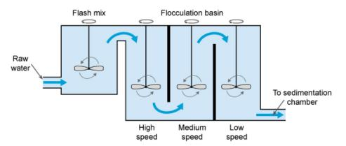
Figure 5.5 The coagulation–flocculation process.
