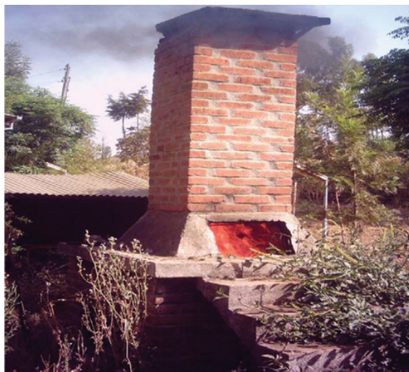
Figure 10.5 (a) A metal incinerator with a chimney. (b) A brick incinerator is simpler and cheaper to build.
