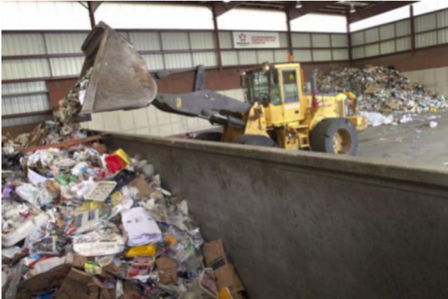
Figure 9.5 Mechanically loaded transfer station.
