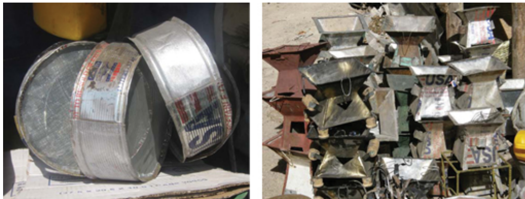
Figure 8.3 Large metal containers can be cut and reformed into new products like these sieves and stoves.
