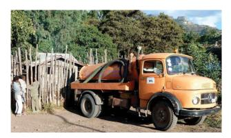
Figure 7.4 A tanker pumping out sludge from a septic tank.
