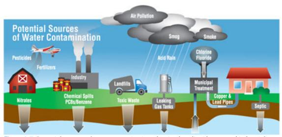
Figure 2.7 Potential sources of water contamination, showing how liquid waste and industrial waste can cause pollution of groundwater and surface water sources (Andrews, 2015).
