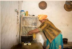
Figure 13.5 This cooking stove is fuelled by biogas.
