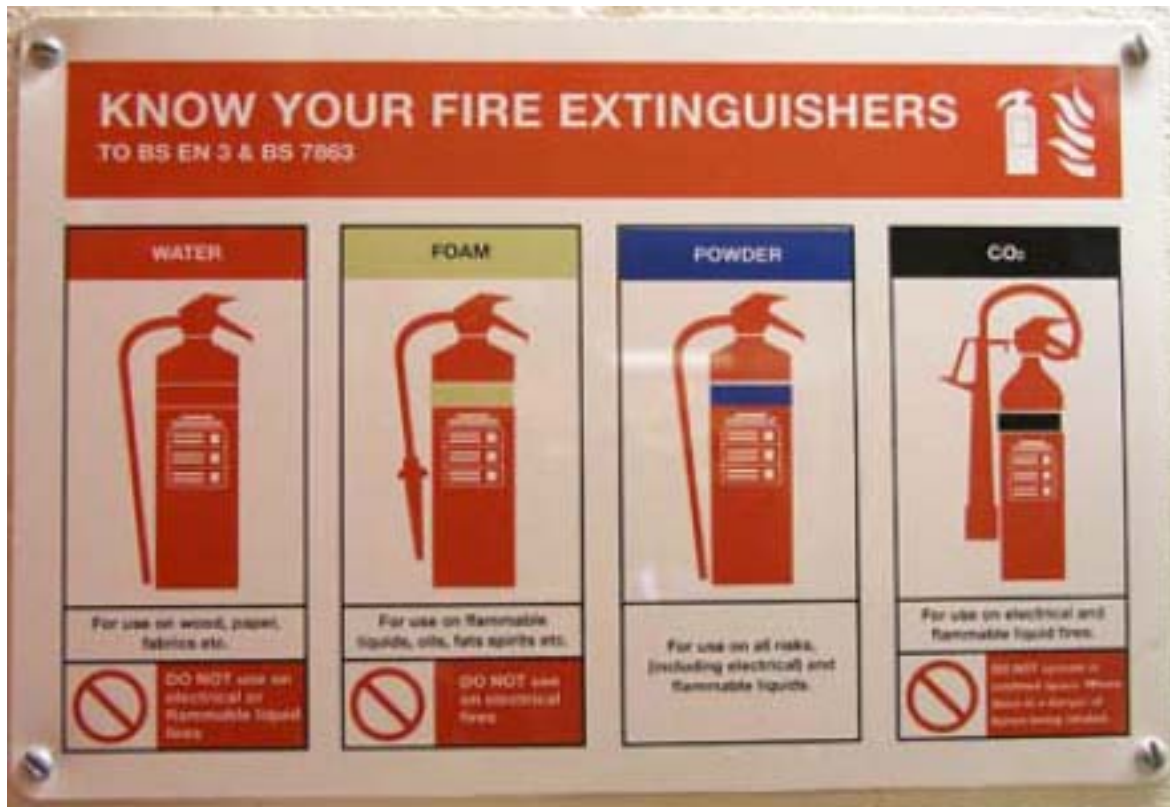
Figure 10 Fire extinguisher symbol chart
