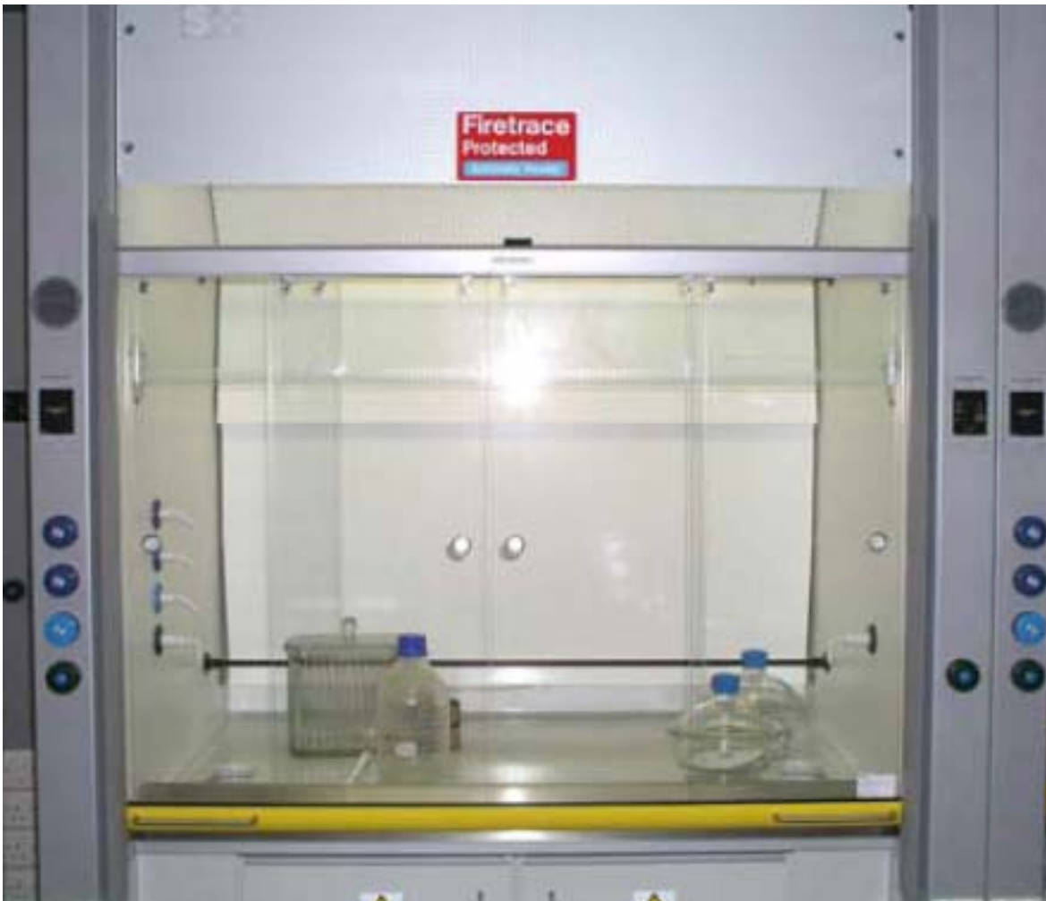
Figure 6 A fume cupboard
