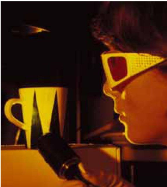
Figure 8 A fingerprint on a mug has been made visible in fluorescent light. To see the fluorescence clearly it is necessary to work in a dark room using UV light. To avoid damage to eyes from the UV radiation, protective goggles need to be worn.
