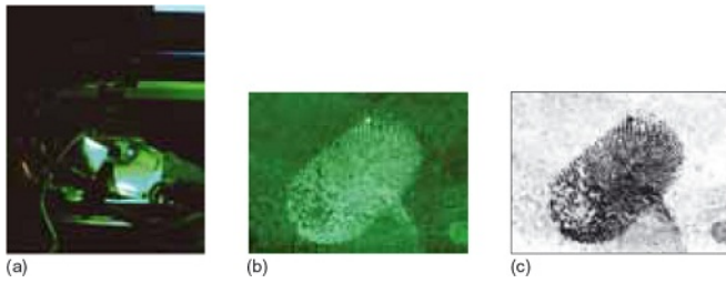
Figure 4 Fingerprint on a vehicle bonnet photographed and enhanced using the DCS-3 system. (See text for details.)
