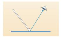
**Figure 6** Reflection of light. If white light is directed onto a blue material, all the wavelengths apart from blue are absorbed by the blue dye. The blue light is reflected.
