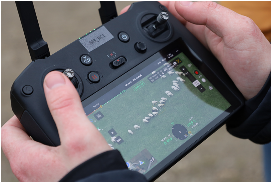
Figure 8 A drone hand-held controller with high resolution screen, allowing for close inspection of individual animals from a distance. With such level of detail, drones are worthy of their 'nickname': 'an eye in the sky'. Picture taken during a drone demonstration event led by Adrien Lebreton, at CIIRPO farm, IDELE's sheep research facility, Massif Central, France
