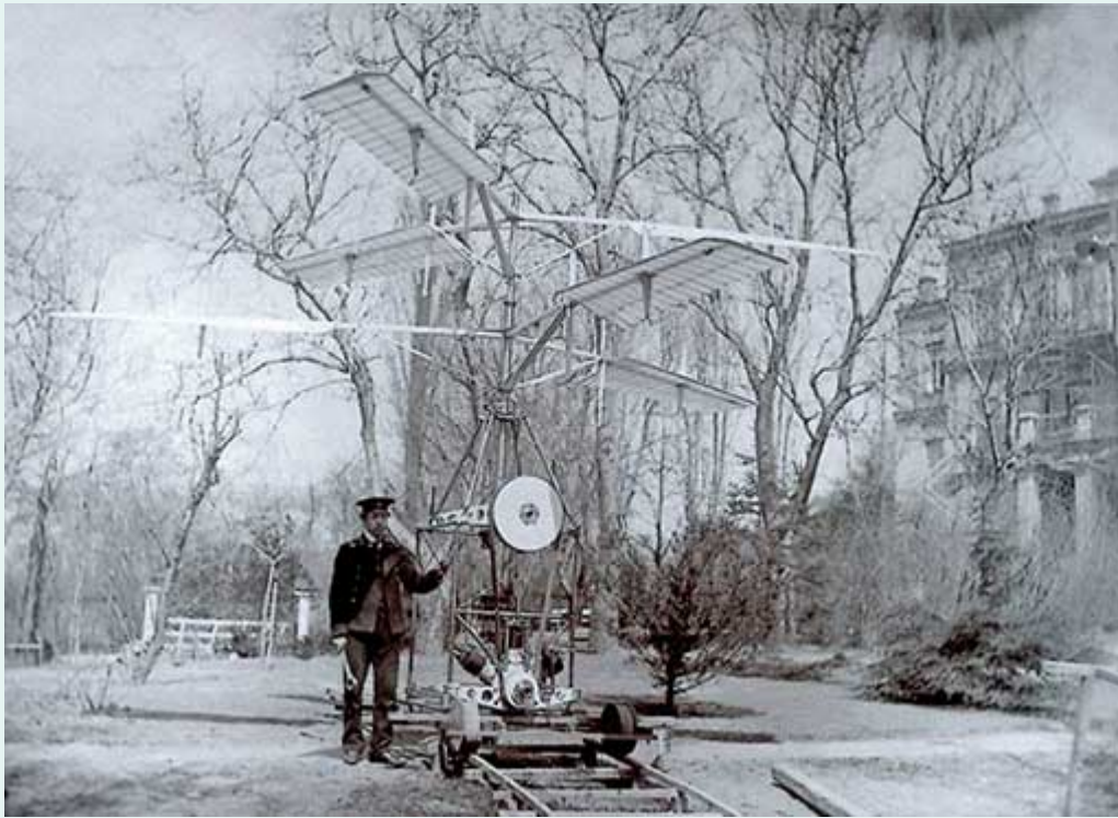
Figure 5 Igor Sikorsky's 'H2' helicopter (1910)
