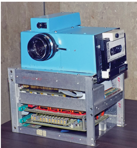
Figure 16 An early Kodak prototype of a digital camera, circa 1975.
