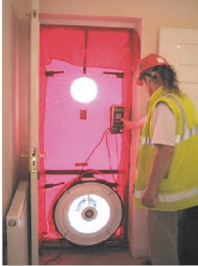
Figure 18 A blower door being used to pressurise a house to test its airtightness (courtesy Leeds Metropolitan University)
