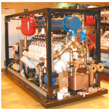
Figure 35 A small- scale CHP unit before installation; the engine is at the front and the generator at the rear (courtesy of Cogenco)
