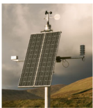
Figure 2 A roadside weather monitoring station. Note the anemometer at the top for measuring wind speed, and the characteristic photovoltaic panel, which recharges the station battery to power the instruments.
