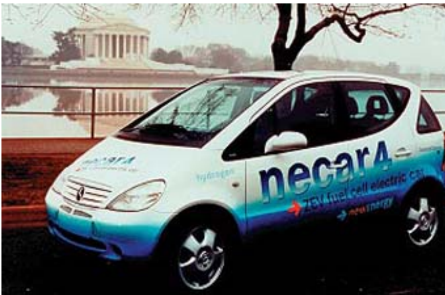
Figure 54: This Mercedes A-Class car is powered by a fuel cell running on hydrogen. The manufacturers, Daimler-Chrysler, and other car-makers such as Ford and General Motors, have announced plans to introduce similar cars on the market
