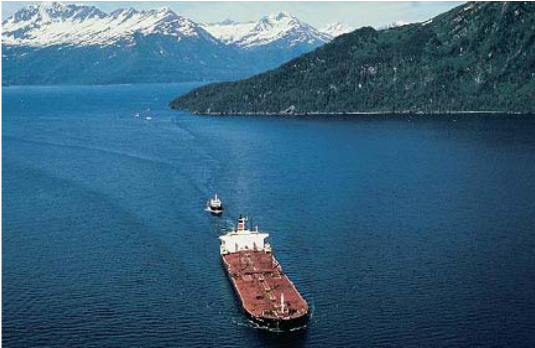
Figure 11: A typical supertanker used to ship oil around the globe. To transport the c.3500 million tonnes of oil used by the world in 2000 would require some 14,000 tanker journeys, assuming a typical tanker capacity of 250,000 tonnes. Total world primary energy use in 2000 was equivalent to the capacity of some 40,000 supertankers of this size
