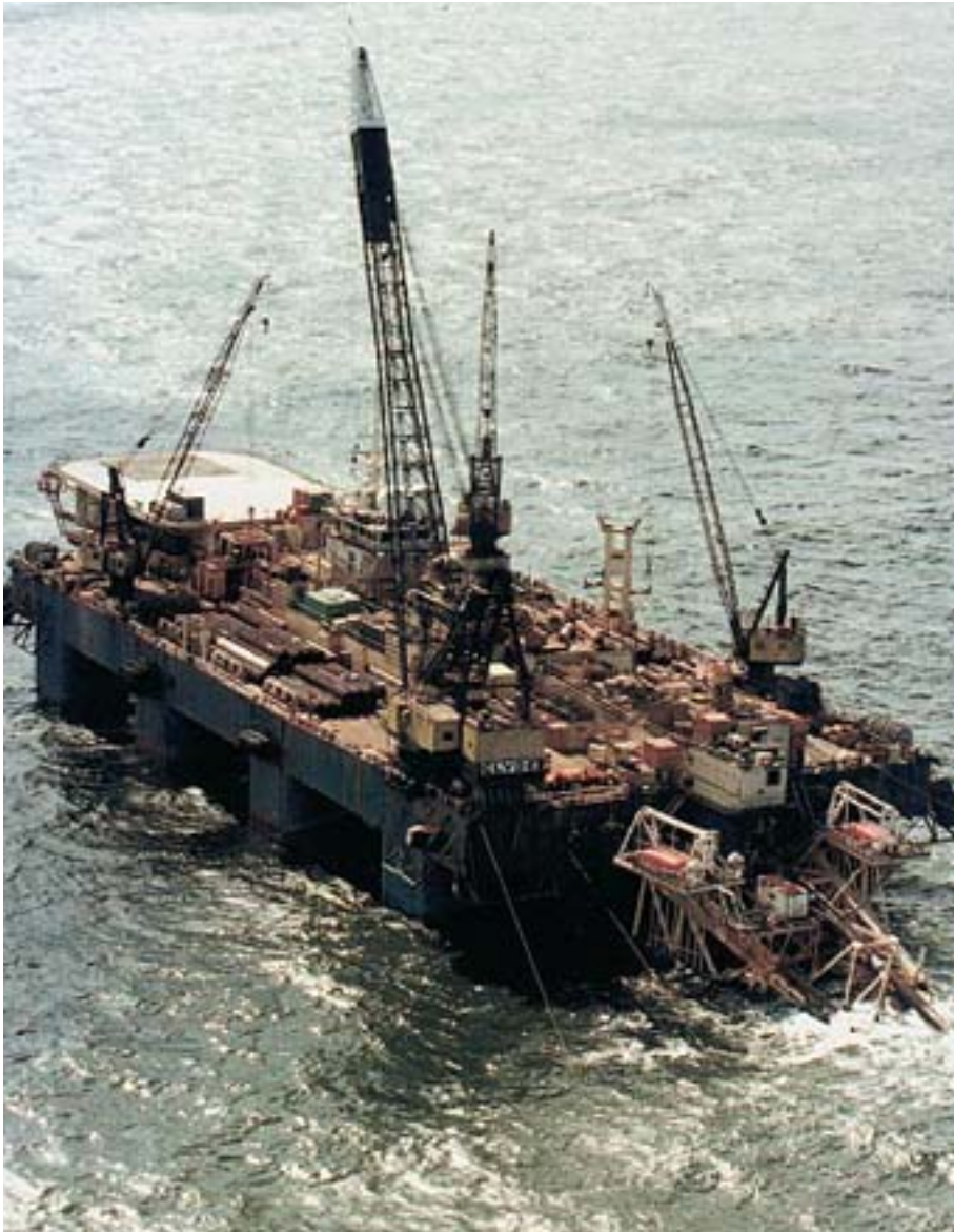
Figure 15: The offshore rig Semac 1, a natural gas pipelaying barge in the North Sea
