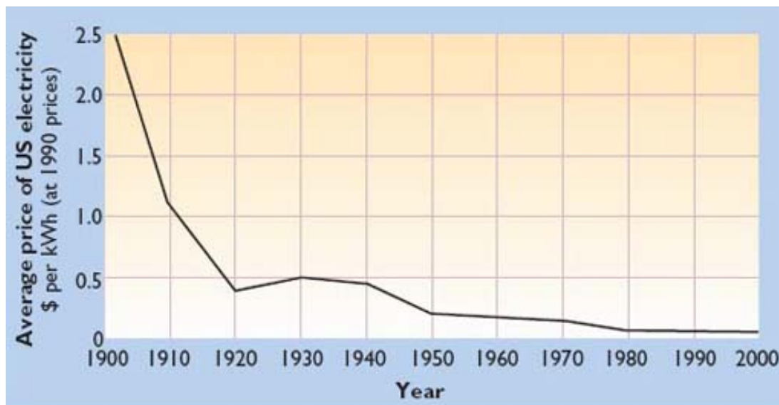
Figure 42: Average household rates for US electricity, 1900–2000, expressed in real terms, i.e. taking into account the effects of inflation (source: Smil, 2000)
