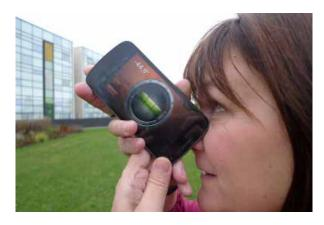
Using a mobile phone tilt sensor to measure the height of a building
