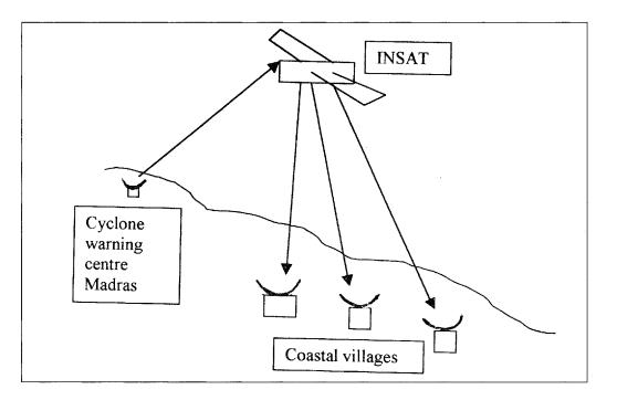
The satellite sends a code to receivers in the appropriate village, which triggers a warning siren. These receivers work continuously and are powered by solar cells.
