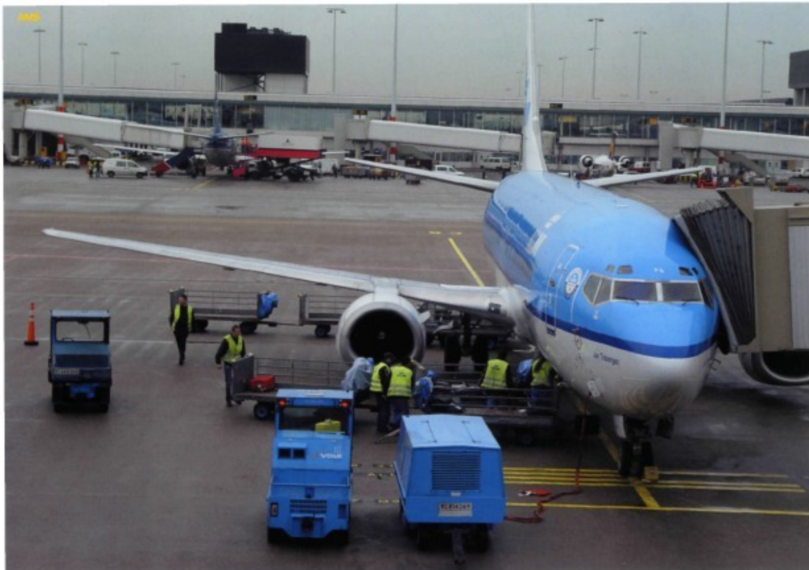
Mobile generators (GPUs) provide power to planes while they are on the tarmac.
