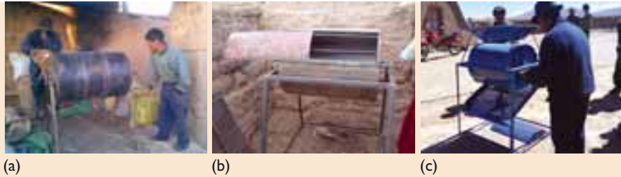
Figure 11.7 Three different potato peelers. (a) Peeler machine first model; (b) peeler machine second model; (c) peeler machine final model
