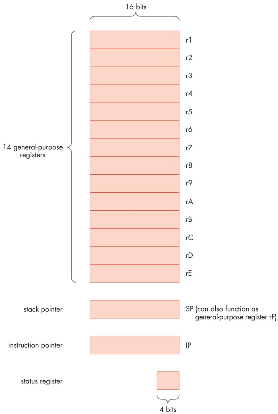
**Figure 1** The programmer's model of the simulated processor
