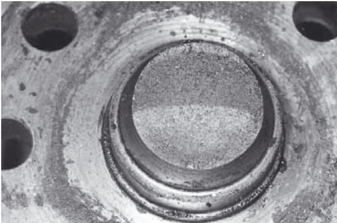
*Figure C17* Brittle fracture in cast-iron
