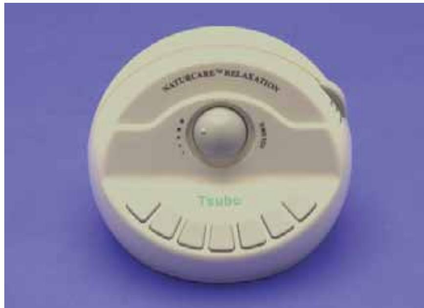
**Figure 9** Environmental sound generator used in sound therapy for tinnitus.
