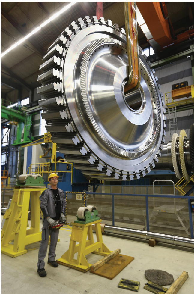
Figure 25 Worker with a disc for a gas turbine at the Siemens manufacturing plant
