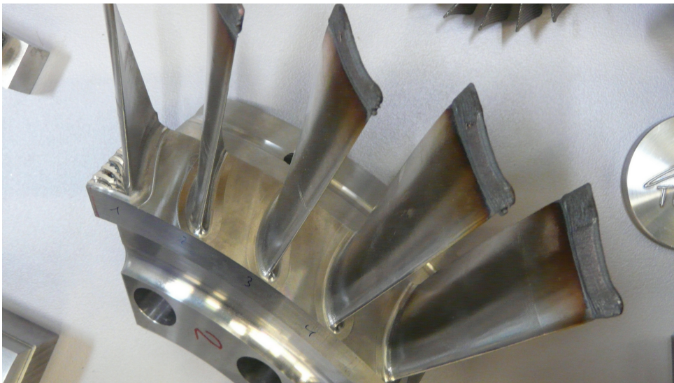
Figure 5 Gas turbine blades with tip repairs
