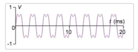
Figure 27 Combination of two sine waves
