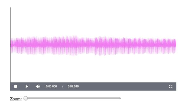
Figure 19 Voltage wave produced by humming a low note
