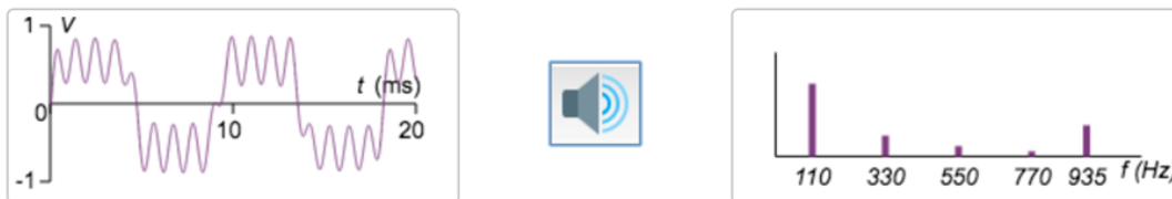
Figure 31 Noise with frequency f = 935 Hz shows clearly in the frequency domain
