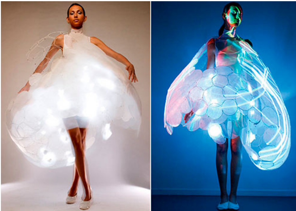
Figure 8 The Bubelle Dress from Philips Design features sensors embedded in its inner lining that monitor the heartbeat of the wearer, which is translated in lighting effects on the outer layer visible to others
