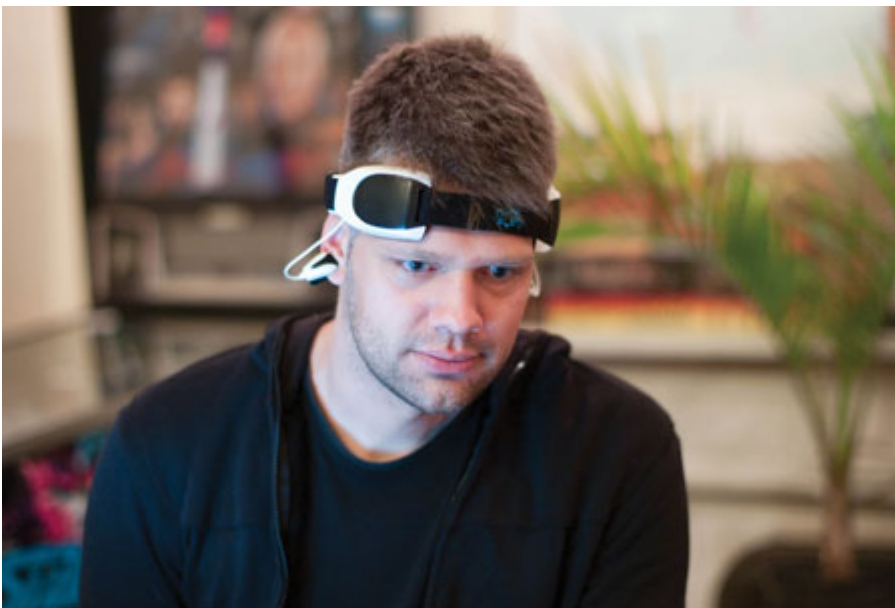
Figure 6 User playing the computer game 'MindFlex' wearing a special EEG headset which captures brainwaves and enables the player to steer a small ball through an obstacle course
