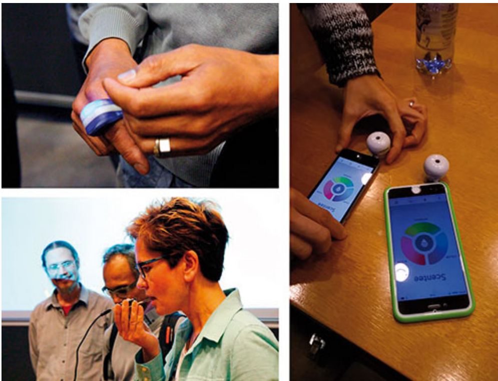
Figure 15 The devices pictured were developed at the Mixed Reality Lab based at City University London. Each uses a different sense to communicate remotely: the device on the top left is a ring that vibrates when the receiver is being kissed by the sender; the device on the right can be connected to a smartphone to receive scent messages from a sender; the device on the bottom left enables the user to receive messages through taste.
