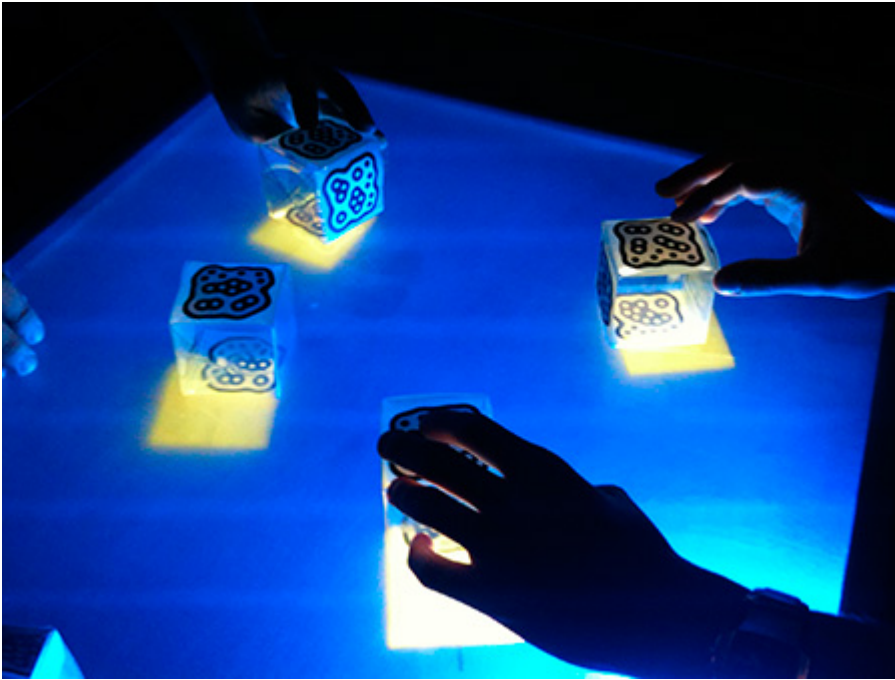
Figure 5 Users making sounds via a musical tabletop by manipulating and moving digitally enhanced cubes on its surface
