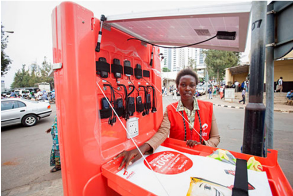
Figure 11 A Mobile Solar Kiosk, which provides low-cost, solar-powered phone charging to users in Rwanda
