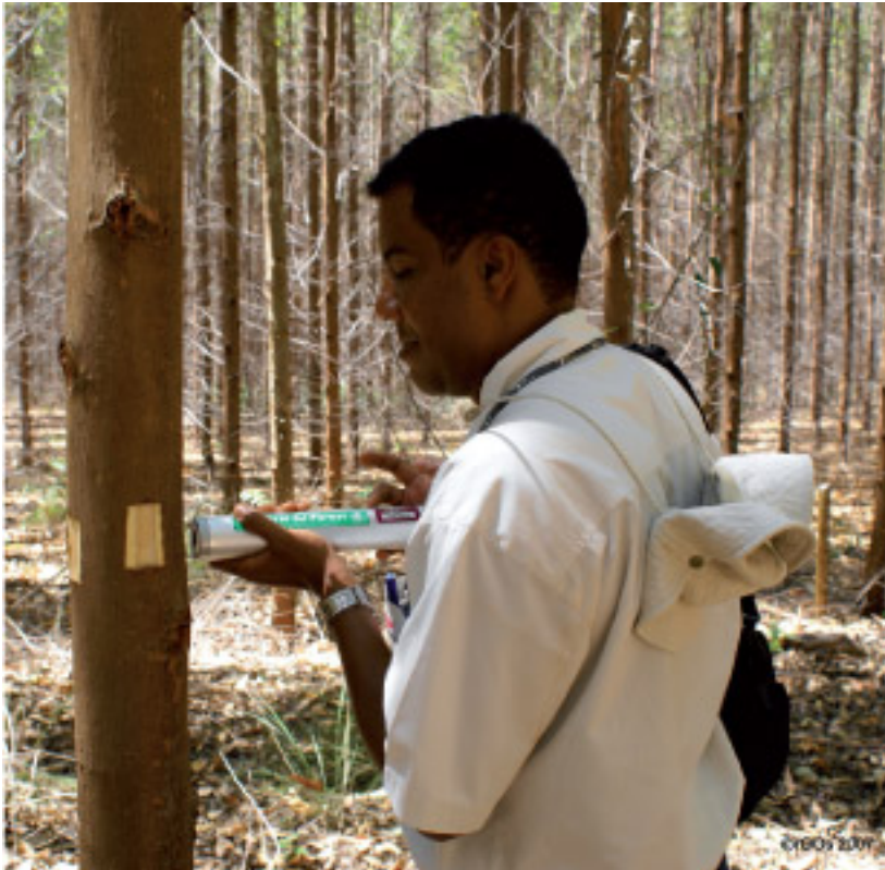
Figure 8 A pilodyn being used for testing. The instrument is placed up against the wood, and then the pin is fired.
