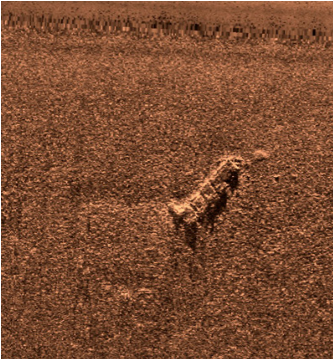
Figure 3 Sonar image of HMS Impregnable obtained by side-scan survey.
