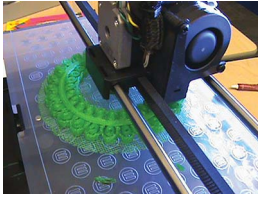
Figure 1 A 3D printer producing a plastic bracelet.
