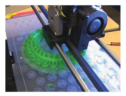
Figure 1 A 3D printer producing a plastic bracelet.
