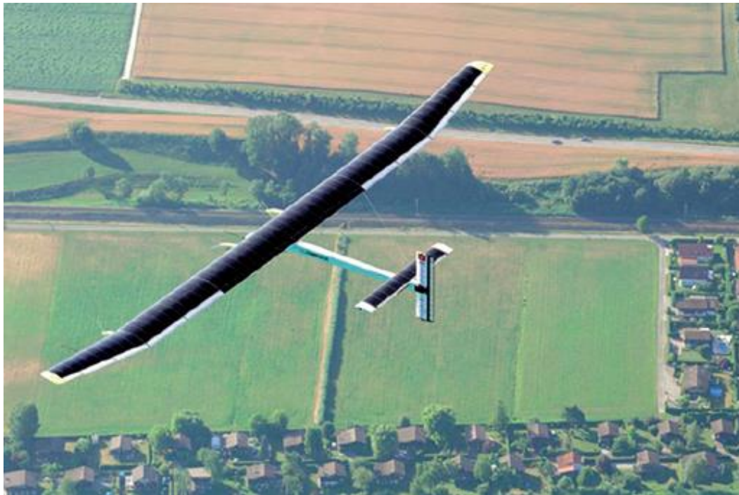
Figure 17 The Solar Impulse, a PV-powered single-seater aircraft. (Solar Impulse, 2011b)
