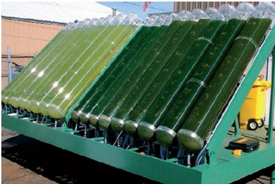
Figure 8 A possible bioreactor design for use of microalgae as an energy source
