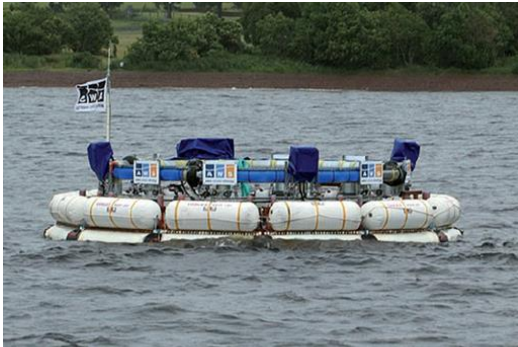
Figure 18 AWS-III in 1:9 scale test on Loch Ness, Scotland
