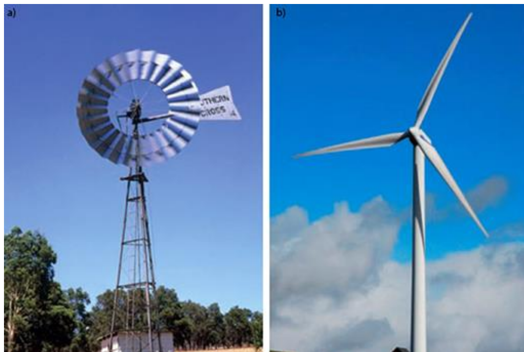
Figure 3 a) Multi-bladed wind powered water pump b) Three-bladed HAWT (Vestas V52 850 kW turbine)
