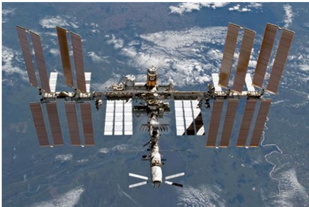
Figure 1 The International Space Station is powered by large arrays of solar photovoltaic panels with a combined output of around 130 kW
