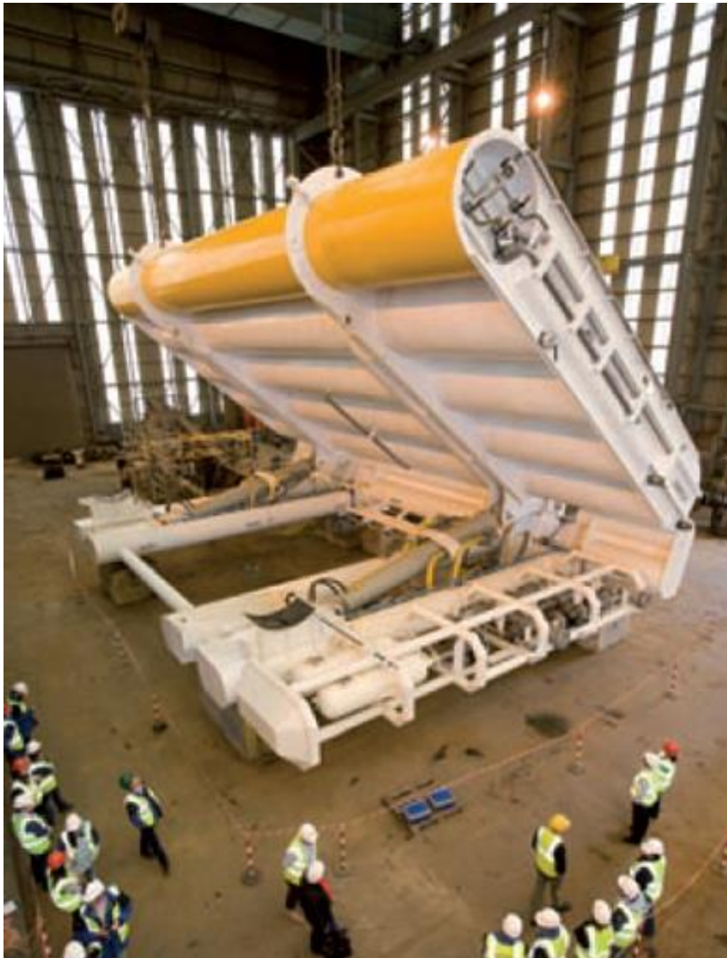
Figure 15 The 315 kW Oyster I in the factory
