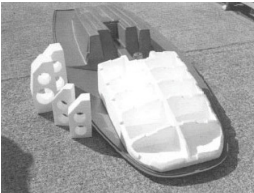
Figure 70 Foam interior to front deck to improve compressive stiffness against point loads.
