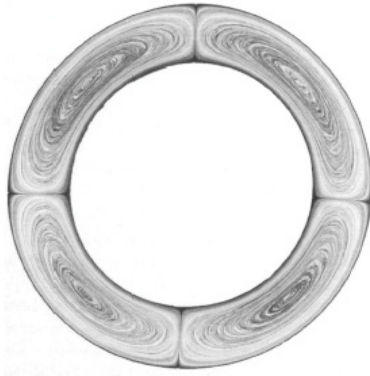
Figure 52 Thin slice of part of a PE tube 5 cm outer diameter (o.d.) showing the poor distribution of carbon black masterbatch during extrusion. The carbon black is added to give protection from sunlight but because of poor mixing can weaken the product substantially. The quadrants are created by spiders in the extrusion head which divide the mixing polymer melt. Source: RAPRA
