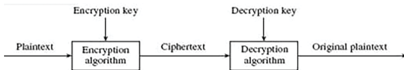
Figure 4 Encryption and decryption
