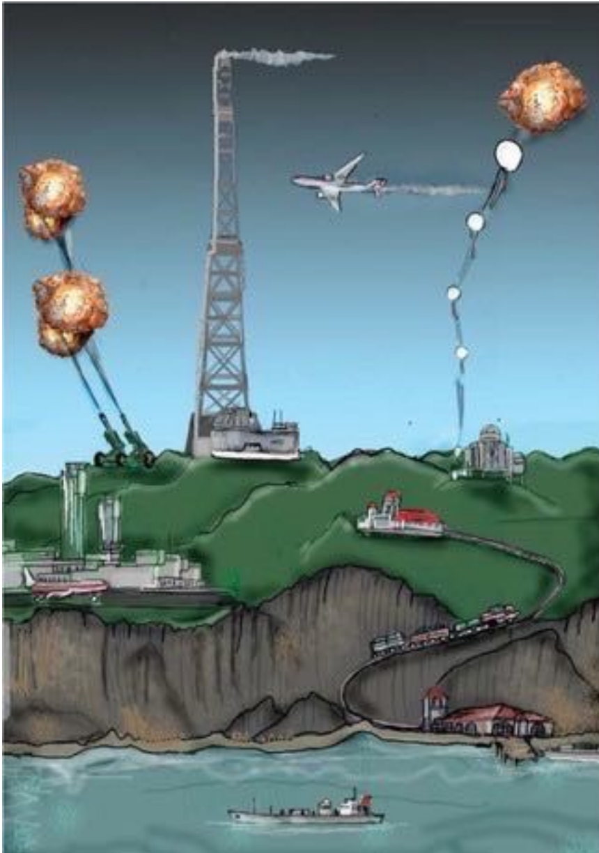
Figure 6 Proposed methods of stratospheric aerosol injection – artillery shells, a tall tower, aeroplanes and balloons – on a mountain, with supplies arriving by train.
