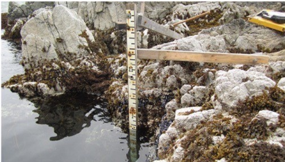
Figure 11 Tide staff used by NOAA 'Teachers at Sea' Rosalind Echols and Avery Marvin to check against tide gauge data while surveying the ocean floor off Alaska.
