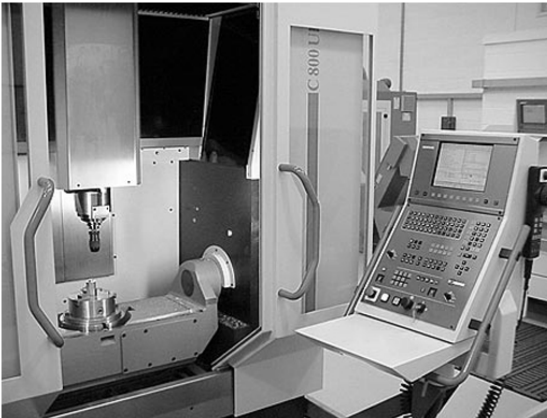
Figure 41 Typical computer-controlled machining centre
