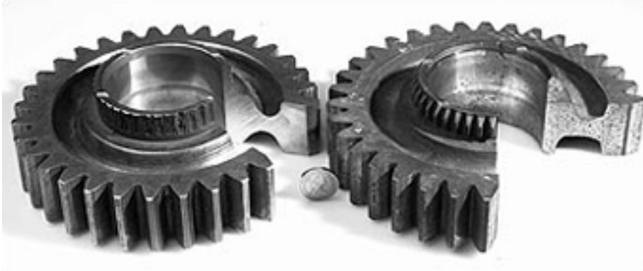
Figure 38 An unused gear (on the right) showing the ring of teeth which were breaking off – the smaller teeth at the top of the gear. The gear on the left was a used gear where the teeth have been worn away.
