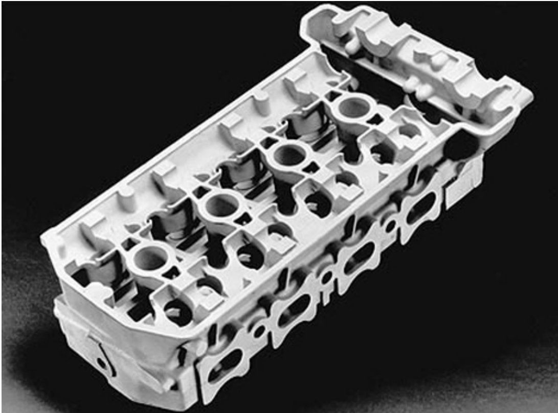
Figure 21 Sand cast (a) cylinder head (b) oil rig joints
