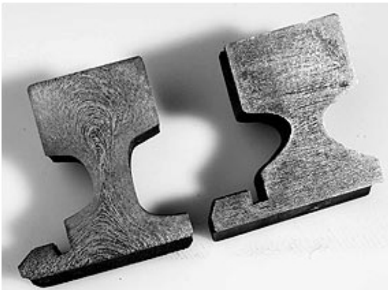
Figure 39 Sections etched to reveal flow lines: (left) original gear, inner teeth worn now; (right) new gear, inner teeth full profile. The teeth are on the bottom left of the cross-sections – compare the sections to the cuts in Figure 38 .
