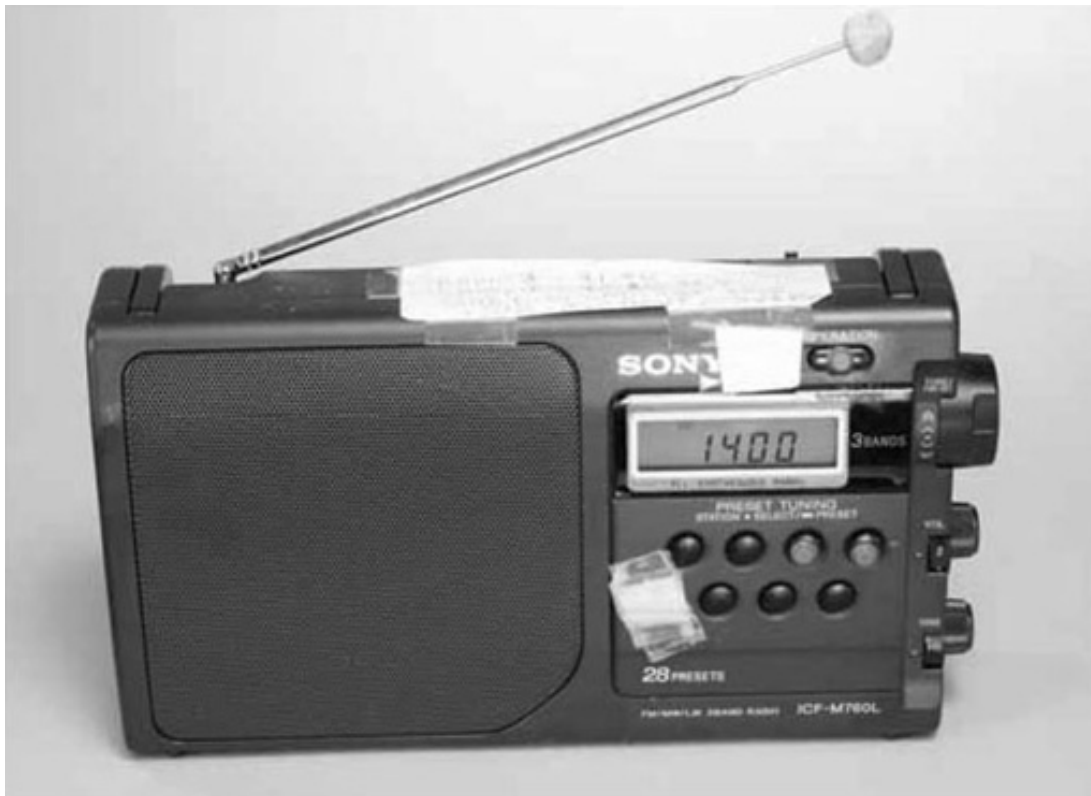
Figure 8 A radio with do-it-yourself adaptations made for a user with poor eyesight and arthritis.
