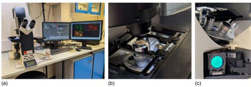
**Figure 7** Inverted fluorescence (light) microscope at The Open University. (a) shows the whole microscope including the computer used to control the microscope and acquire the images. (b) Detailed view of the objectives, placed underneath the sample. (c) Filters that allow for selecting light of a specific wavelength to illuminate the sample.
