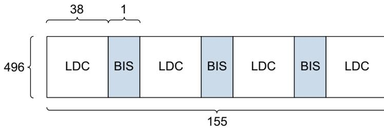
Figure 2.2 Data structure on a Blu-ray disc
