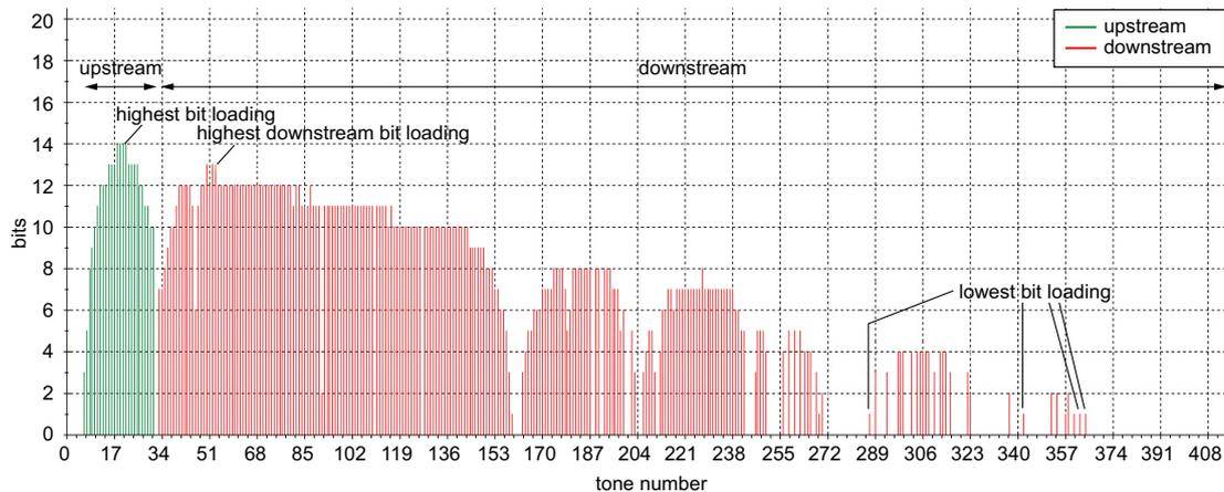
**Figure 4.6 Bit loading of a 2 km ADSL2+ line**
