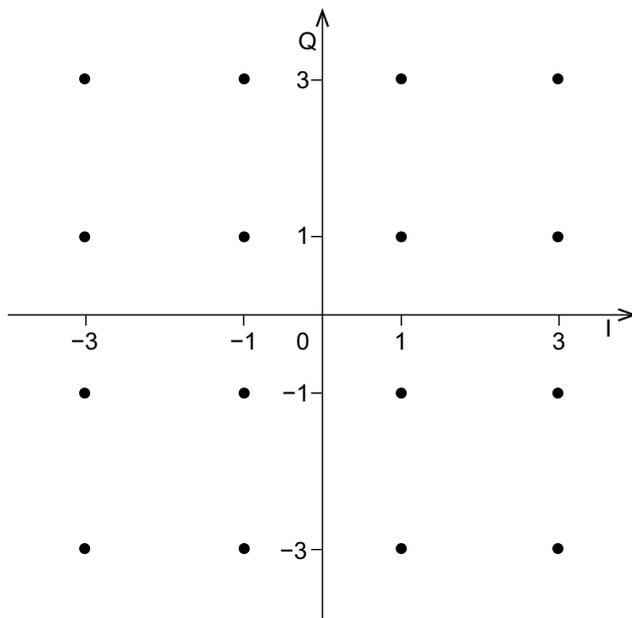
**Figure 1.8 Constellation diagram for 16-QAM.**
