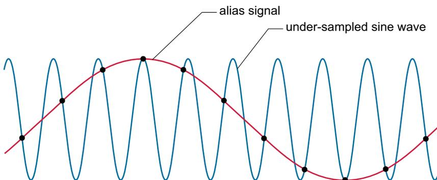
**Figure 3.2** Aliasing of an under-sampled signal
