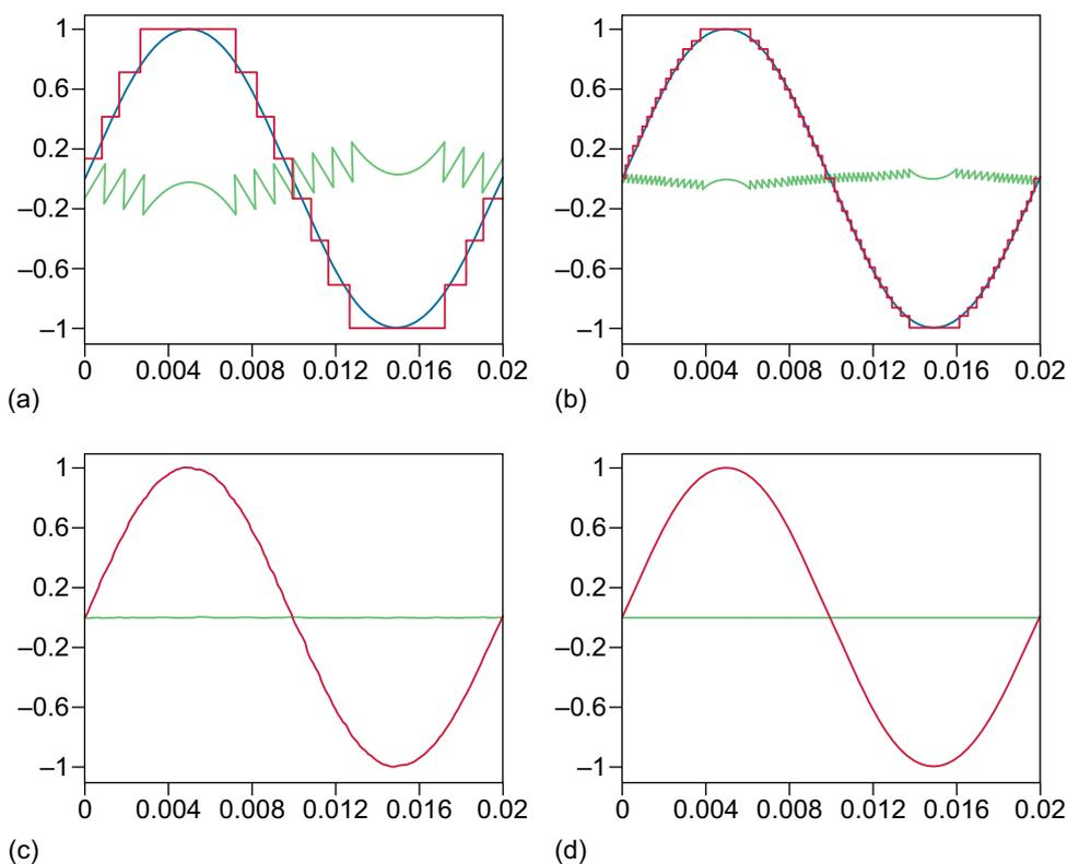
**Figure 3.3** Examples of quantisation error (green) for different ADCs: (a) 3-bit, (b) 5-bit, (c) 8-bit and (d) 16-bit
