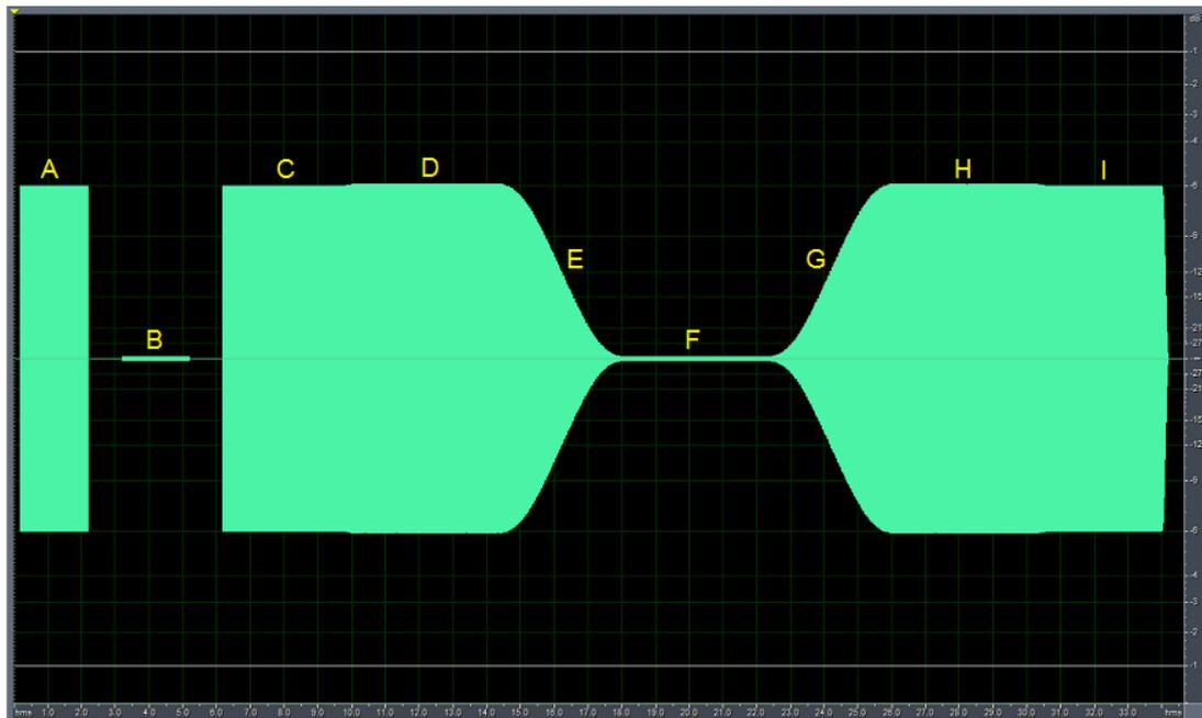
The first two sounds in the clip are simply to familiarise you with the masking tone (440 Hz, shown in the figure at **A**) and quieter masked tone (652 Hz, shown at **B**). You will hear 2 seconds of each.
