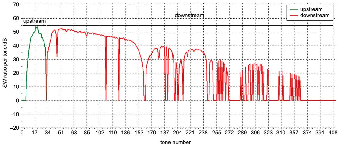
**Figure 4.5 Signal-to-noise ratio of a 2 km long telephone line**
