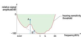
**Figure 3.5** Frequency masking for two single-tone frequencies, A and B, with A louder than B
