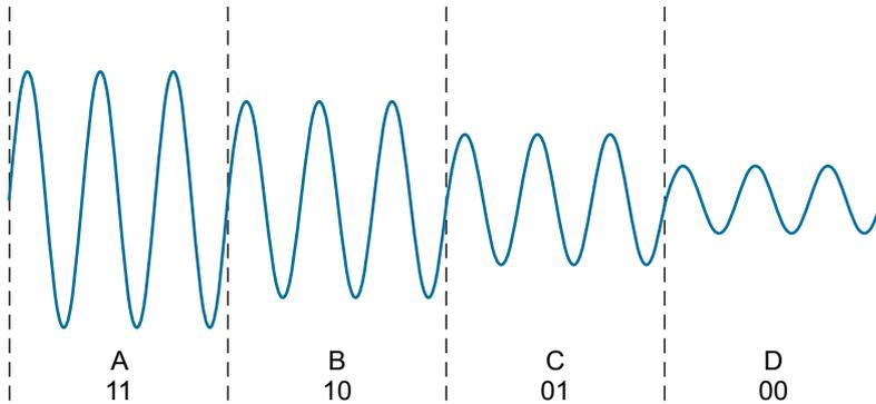
**Figure 1.3 ASK with four amplitude levels**
