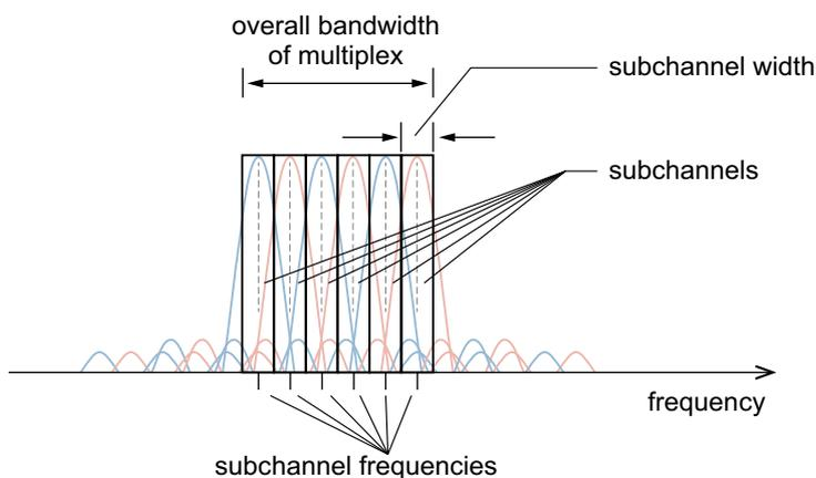
**Figure 4.3 Subchannels centred on subcarrier frequencies**
