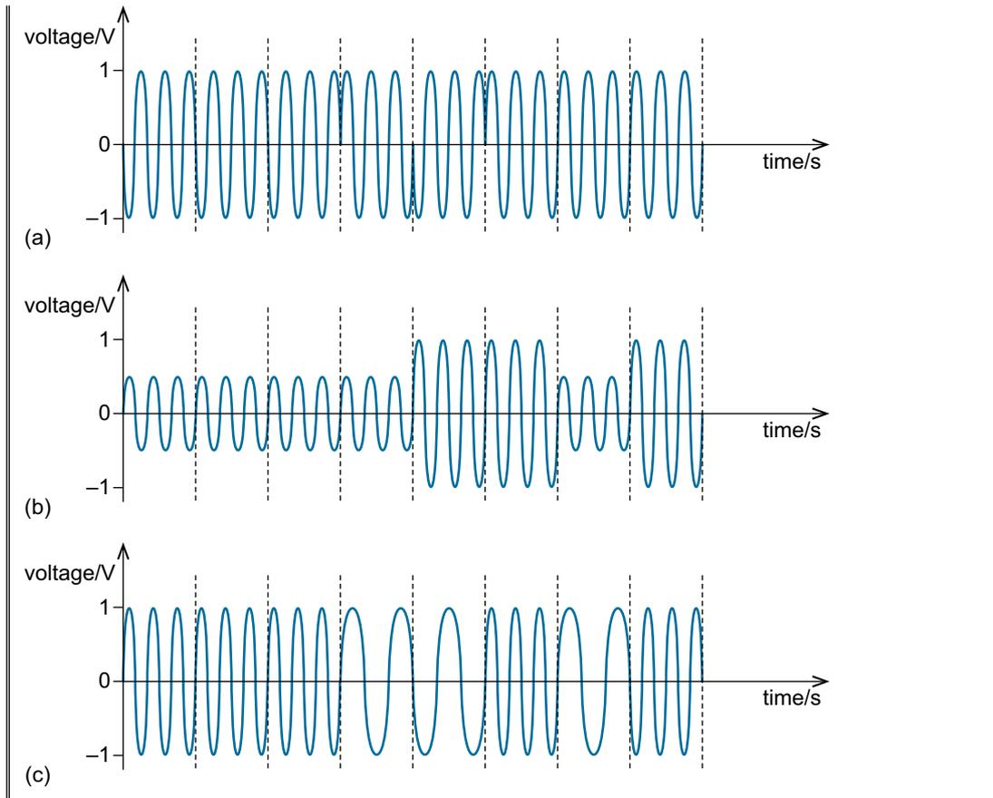
**Figure 1.6** Three digitally modulated waveforms.
