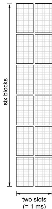
**Figure 4.11 Smallest resource-block allocation in 4G**
