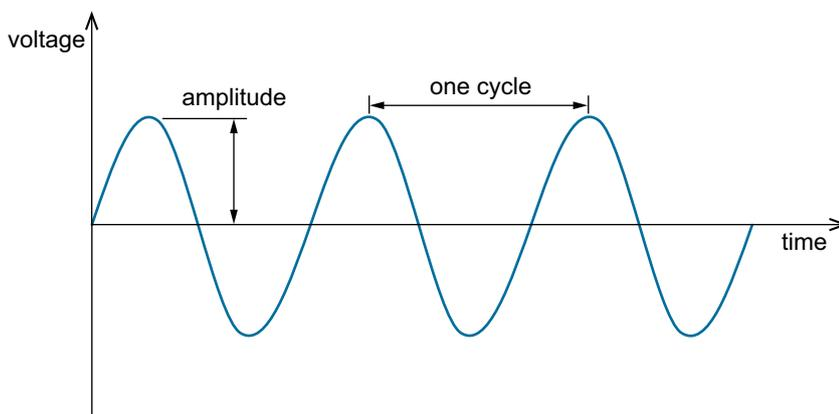
**Figure 1.1 A sinusoidal signal**
