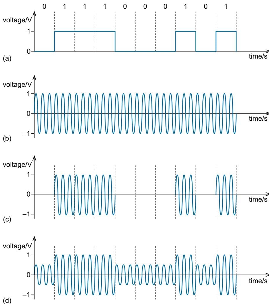
**Figure 1.2 ASK: (a) data; (b) unmodulated carrier; (c) on–off keying (OOK); (d) binary amplitude-shift keying (BASK)**
