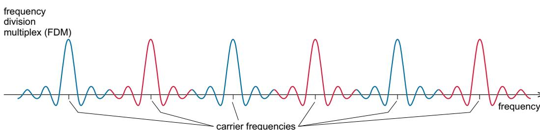
**Figure 4.1** Wide carrier separation in Frequency Division Multiplexing
