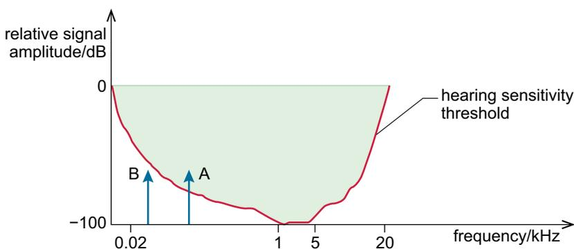
**Figure 3.4** Hearing sensitivity threshold response curve of the human ear with two equal-amplitude frequency tones, A and B
