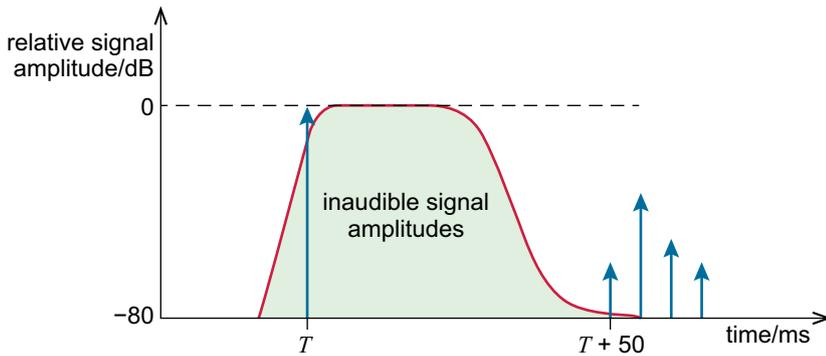
**Figure 3.6** Temporal masking effect of a loud sound at  $T$  and resulting inaudible envelope
