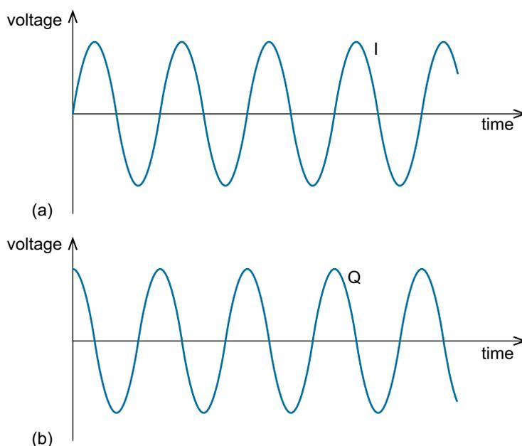
**Figure 1.7 (a) I (in-phase or sine) wave and (b) Q (quadrature or cosine) wave**
