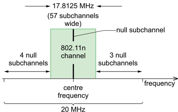
**Figure 4.12 Subchannel nulling used in an 802.11n channel**
