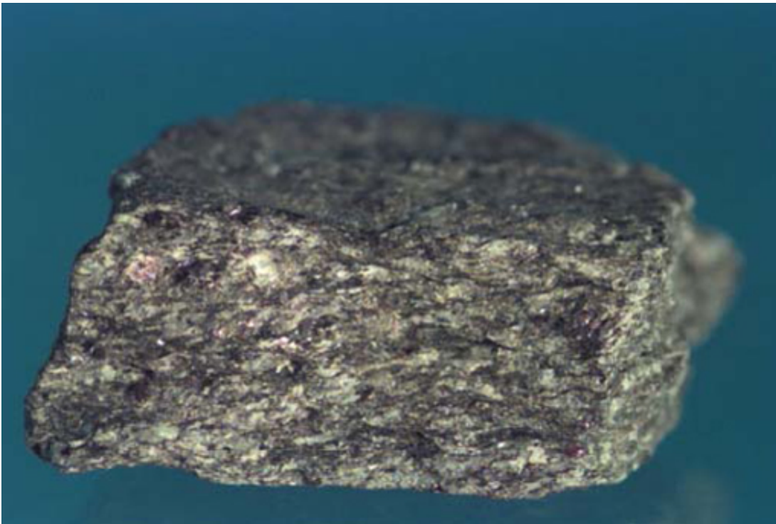
Figure 15 The metamorphic rock schist. The platy mica crystals (dark) are arranged in undulating layers, defining a foliation. The sample is about 6 cm long
