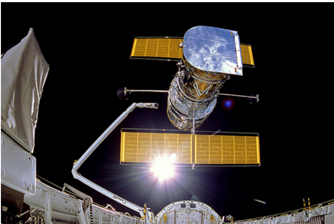
Figure 19 The Hubble Space Telescope being released from the bay of the Space Shuttle
