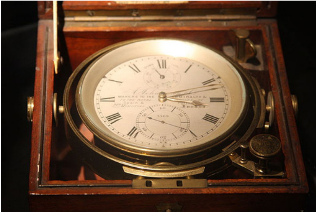
Figure 18 A John Harrison marine chronometer used for establishing the longitude of a ship at sea
