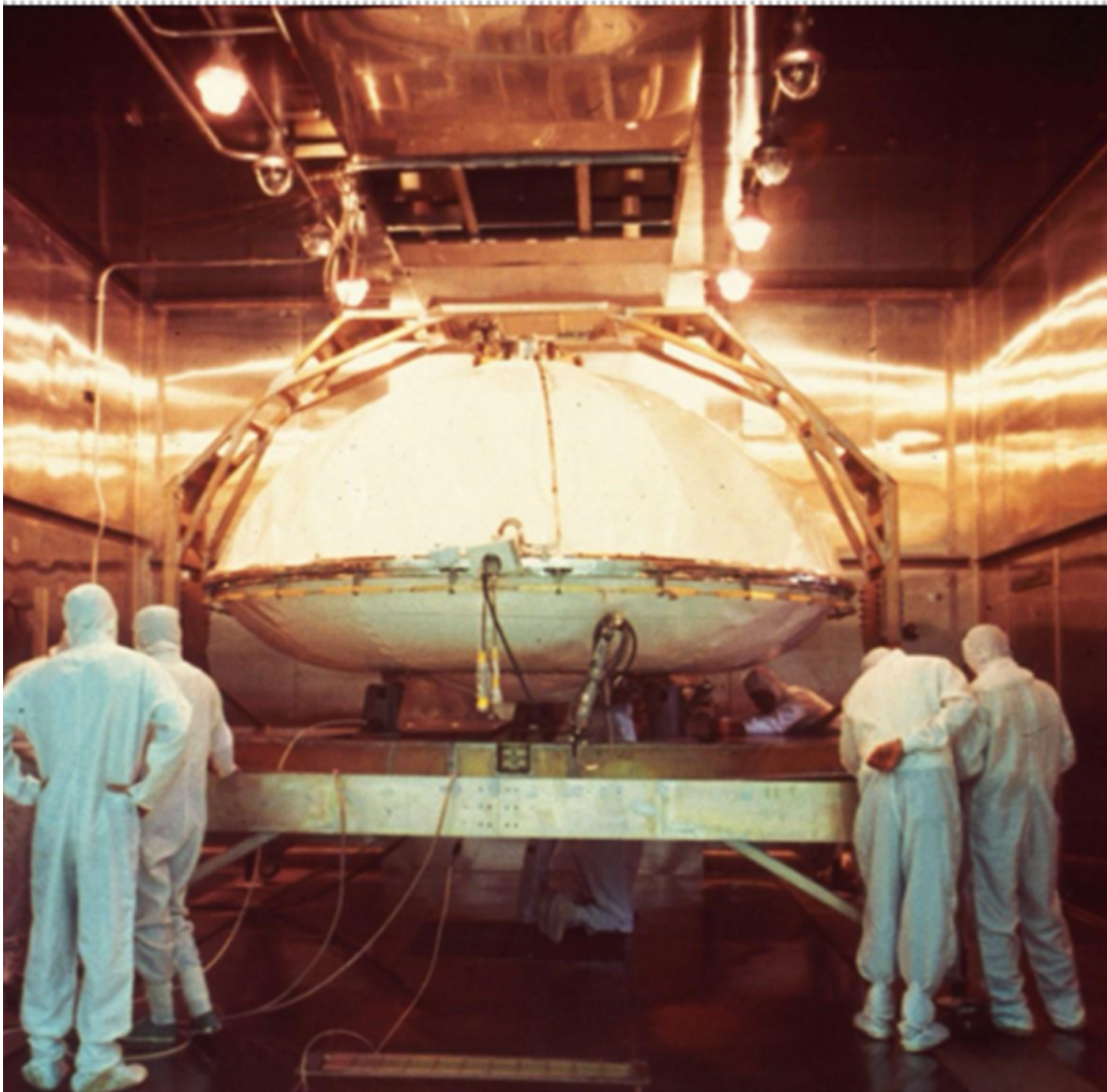
Figure 24 The Viking lander being prepared for sterilisation
