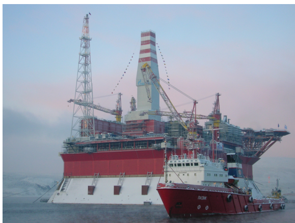
Figure 11 The vast Prirazlomnaya platform, an ice-resistant stationary drilling and oil production platform for use in the Arctic Barents Sea.
