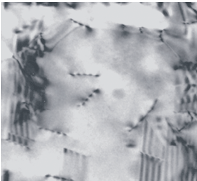
Figure 22 Transmission electron microscope image showing many line defects in a crystal of indium aluminium arsenide (an alloy used in semiconductors). The width of this image is about 1 \mu\text{m} .
