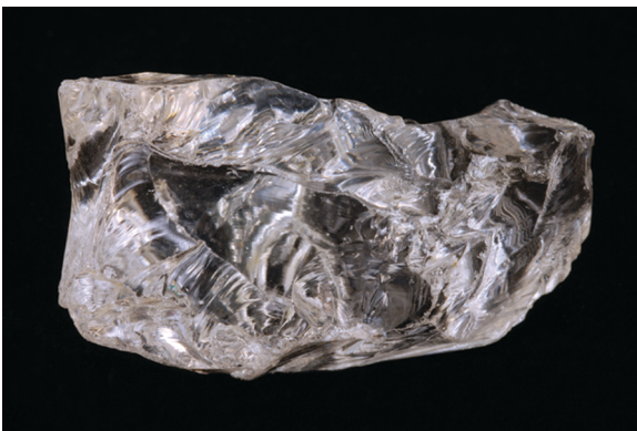
Figure 11 A broken quartz fragment showing an absence of any cleavage planes, and conchoidal fracture (5 cm).
