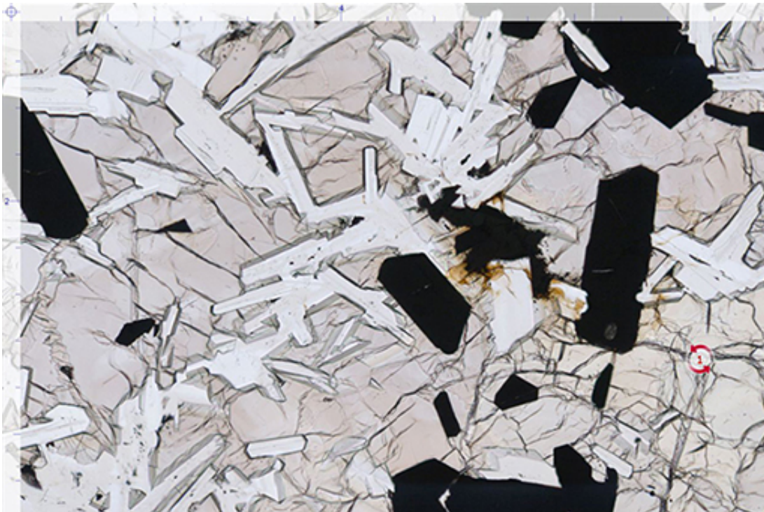
Figure 3 A microscope image of Apollo sample 10029, a mare basalt, taken in plane polarised light.
