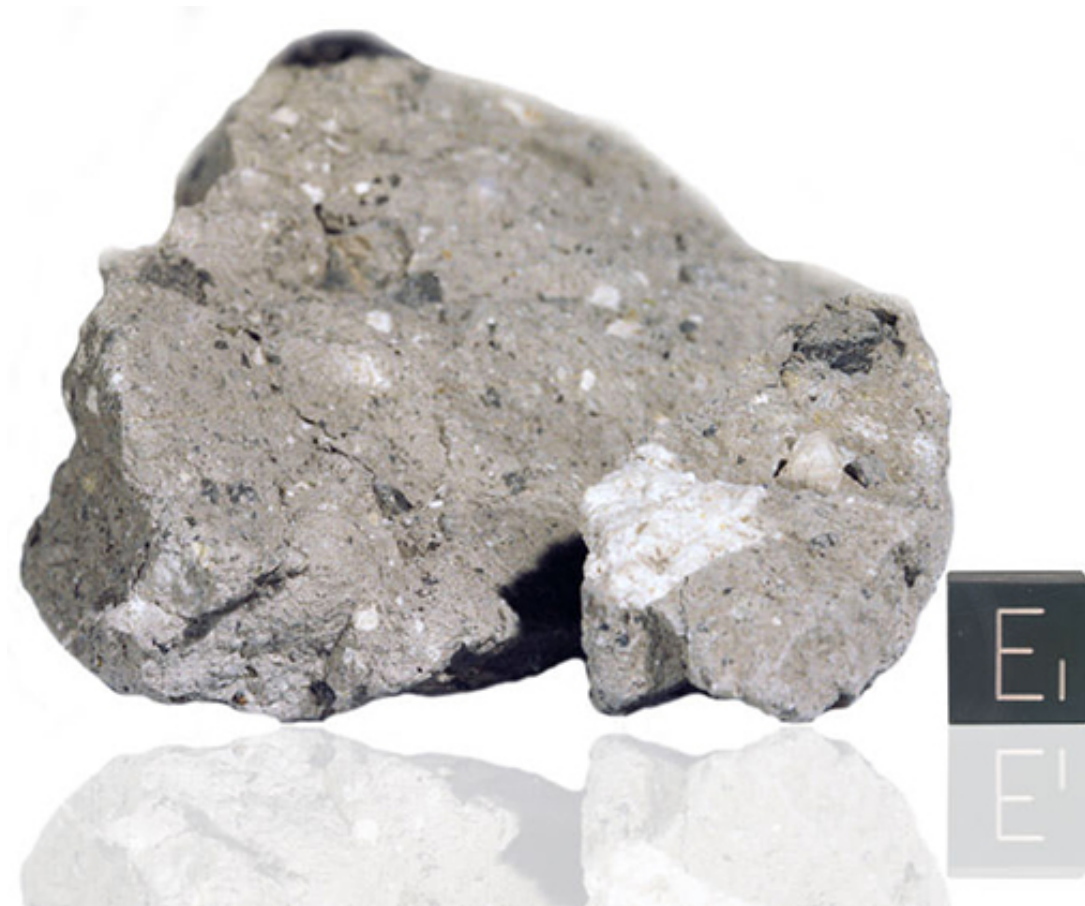
Figure 23 Fragmental feldspar-rich lunar breccia 61295 illustrating the polymict nature of lunar breccias
