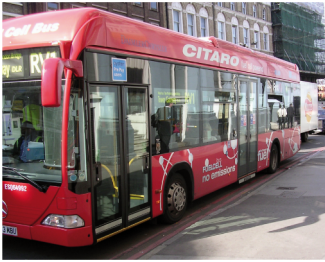
Figure 18 A Mercedes-Benz Citaro fuel cell bus in service in London during the CUTE demonstration (the hydrogen tanks are on the bus roof)
