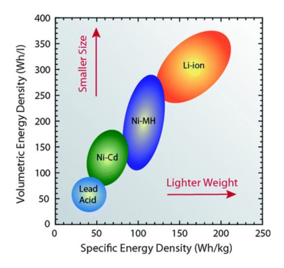
Figure 10: The energy density of different types of rechargeable batteries
