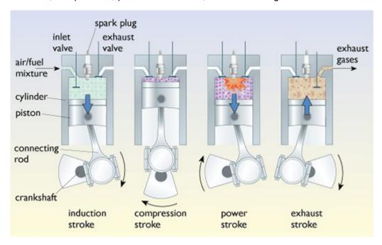
Figure 8: The four strokes of an Otto cycle engine
