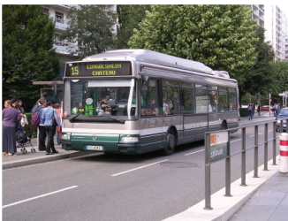
Figure 8 LPG bus in Strasbourg, with fuel tanks on the roof
