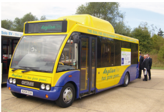
Figure 9 A dual-fuel bus running on gas from a landfill site: originally powered entirely by diesel, the Mercedes-Benz engine has been adapted to run for 60–80% of the time on biomethane
