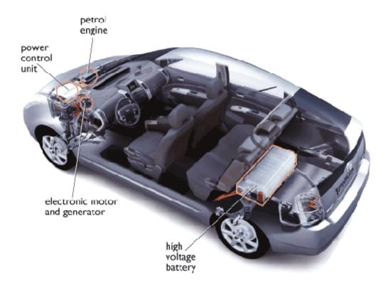
Figure 11: Cutaway section of a Toyota Prius Hybrid
