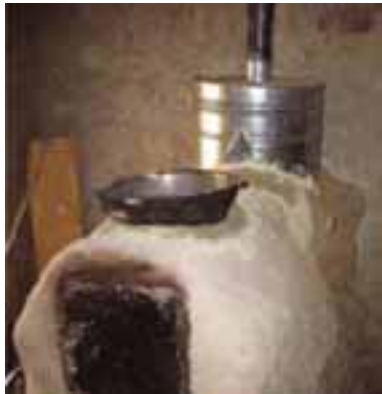
Figure 4.5 A flue attached to an oven prevents smoke and fumes from polluting the air in a rural house. (Photo: Alex Duncan)
