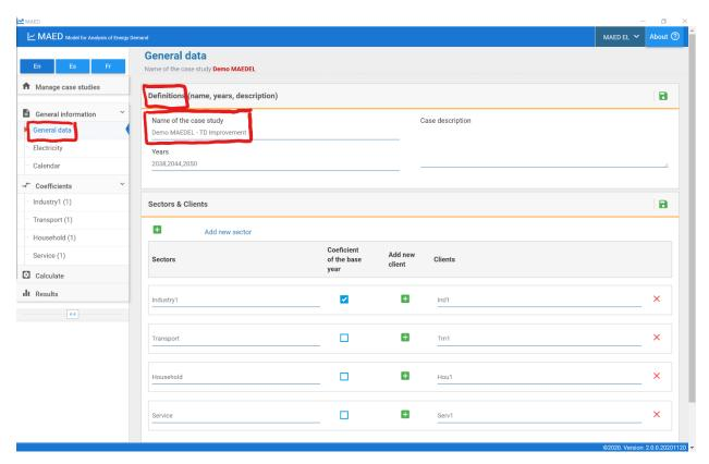
Because all the data from the MAEDEL Demo case study are copied, we only need to change the transmission and distribution losses. Click on the Electricity tab under the General information heading in the navigation menu on the left side of the screen. Click on the Transmission and distribution losses tab at the top of the page. Change the input data as follows:
