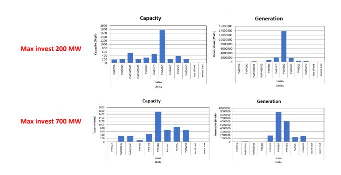
If increased level of Max investment for different technologies affected the role and value of different technologies. In this case, the Nuclear and Hydro replaces geothermal in supplying the base load and geothermal generators are used to supply intermediate and peak loads.
