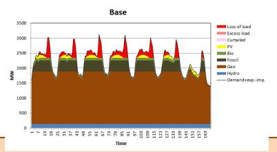
It is evident from the dispatch profile that the availability of solar power is already aligned with the power demand, and also all the units are running at almost full capacity (No curtailments). Therefore the main issue seems to be insufficient capacity.
