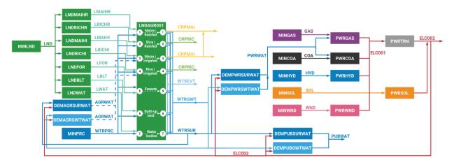
It is essential to notice that the energy input is actually the electricity produced by the power plants. This creates a loop in the model that is essential for capturing the energy links. In this activity, no new technologies and commodities will be added, and all the inputs will be in mode-1
