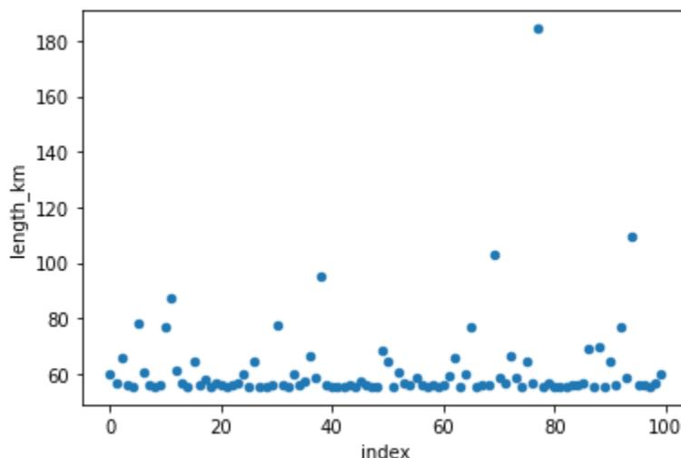
**Figure 7.6:** Scatter plot of route lengths under random failure scenarios.
