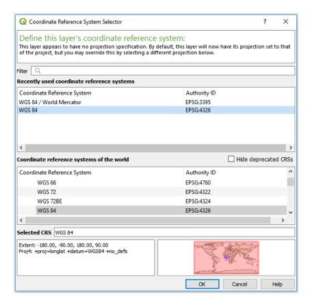
In the filter field start typing the name of the coordinate system you want to use (**UTM zone 31N**) and double click on it as it appears.
