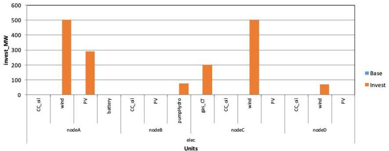
We see that wind power is invested in all allowed nodes. We also see that pumped hydro is invested in in NodeB, as well as additional PV to nodeA.
